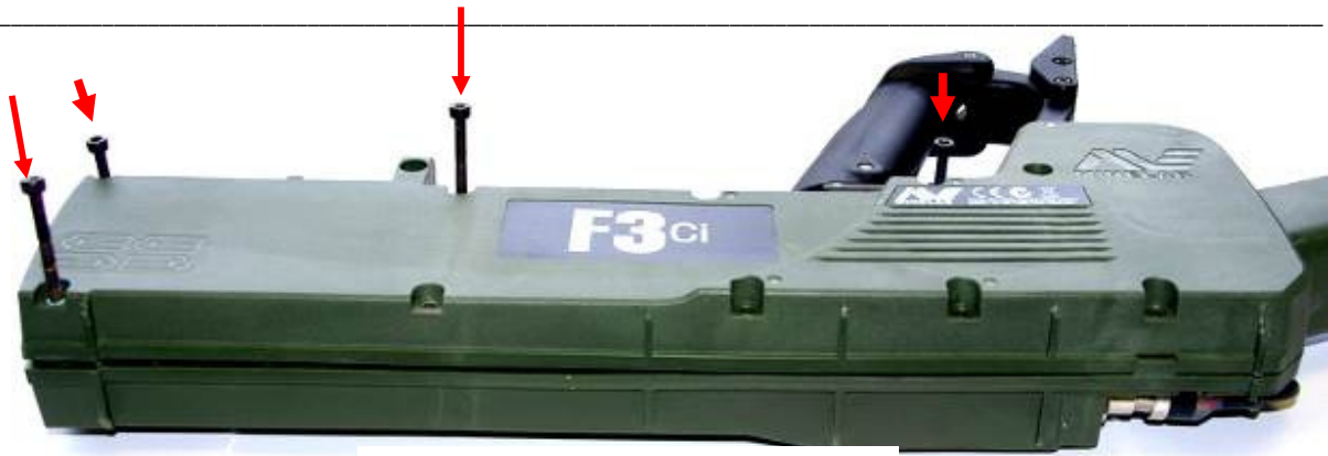
Figure 22: Fitting Four Screws
