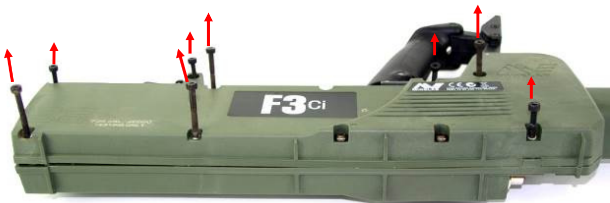
Figure 11: Removing Eight Screws (Allen Key)
