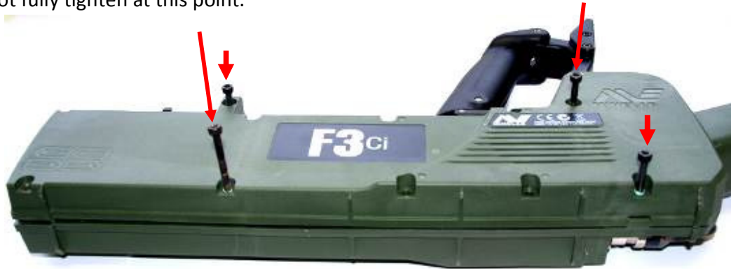
Figure 21: Fitting Four Screws
