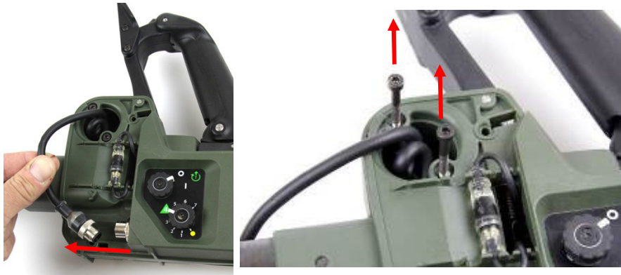
Figure 10: Disconnecting Coil Plug and Removing Screws
