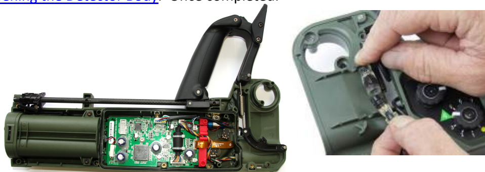
Figure 78: Disconnect Wiring Loom Handle
