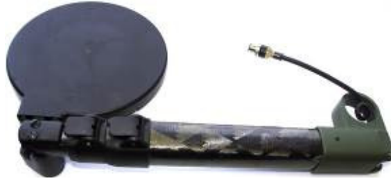
Figure 72: Shaft and Coil removed from Detector
