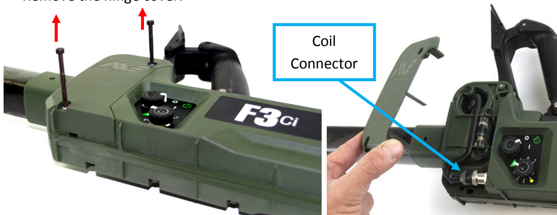
Figure 9: Removing Hinge Cover
