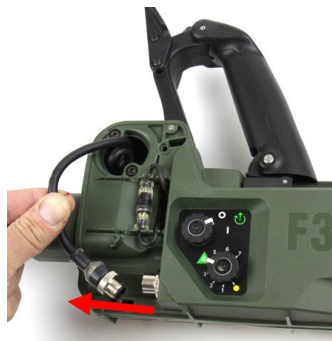
Figure 47: Disconnecting Coil Connector
