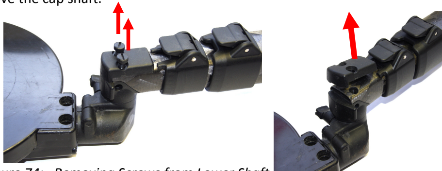
Figure 74: Removing Screws from Lower Shaft
