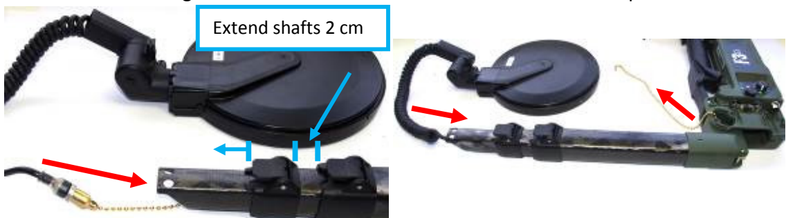
Figure 63: Threading Coil Cable through Shafts
